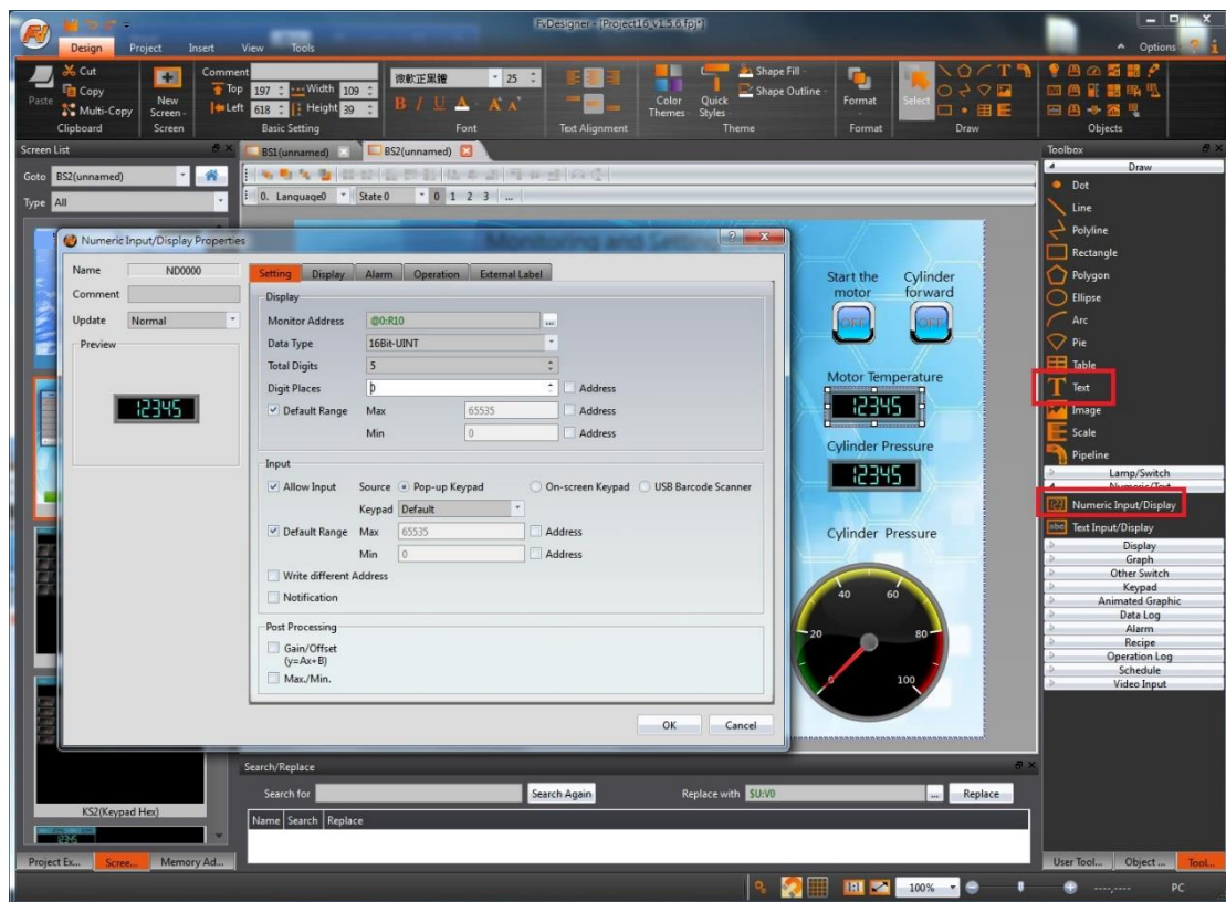
Figure 42 Add text and numeric/input display objects
