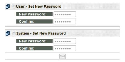
According to operation privilege differences, this product series divides the password section into User password and System password. To enter an operation page, the user password or system password must be entered in order to log in; and to enter the system webpage, the system password must be entered to log in. There is no password set for the default factory user password, and the default factory system password is 1234.
