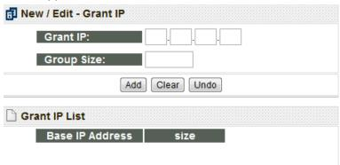
When setting is required, you can fill in the authorization data in the New/Edit-Grant IP field; in the Grant IP field, enter the smallest IP address, and in the Group Size field, enter the number of IPs; click the Add button when completed. To modify or delete an authorization data, click the icons behind the Grant IP List field to perform the operations:
