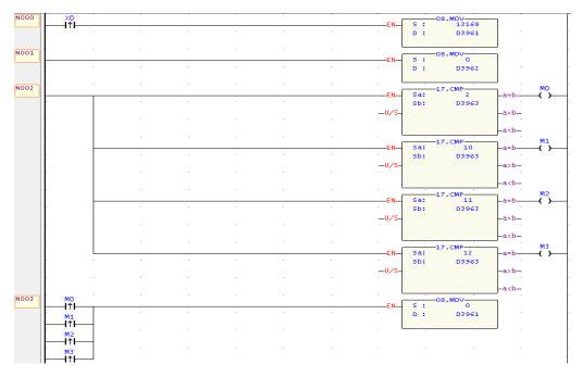
After completing the steps mentioned above, every time X0 changes from 0 to 1, and when D3962 is 0, the mobile phone will receive the SMS.
