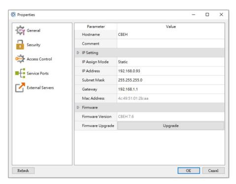
Provides window version setting software for communication modules setting basic configuration, password protection, and firmware upgrade, etc. For more details please refer to ch2.1
