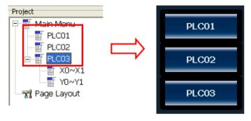
To add a second level sub-menu, just use the mouse and add a new menu in the first level menu just as described above, and as shown below, a sub-menu is added into the first level menu item.
