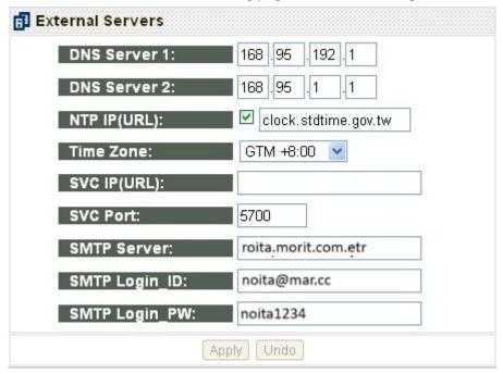
**DNS Server:** Domain name service server. Just like the primary DNS and secondary DNS set on the PC. This setting is not necessary if the network address setting is set to the dynamic (DHCP) mode. The preferred DNS setting in the figure below is the DNS server address of Chunghwa Telecommunications:
