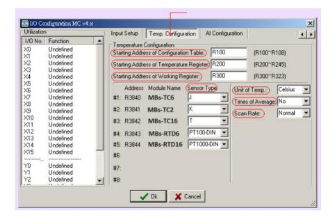
The user need to assign a starting register of a contiguous register area for holding temperature reading value and areas for storing the configuration table and working scratchpad and define the sensor type, unit of temperature, scan speed and samples for average.
