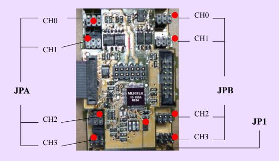
The jumper setting for each type of signal output are shown at below:
