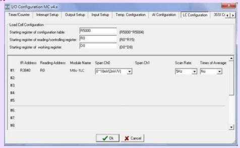
Before MBs-1LC module can be working, the configuration of the module should be set by the Winproladder software tool. The picture shown at above is the I/O configuration page for "LC module" setup.
