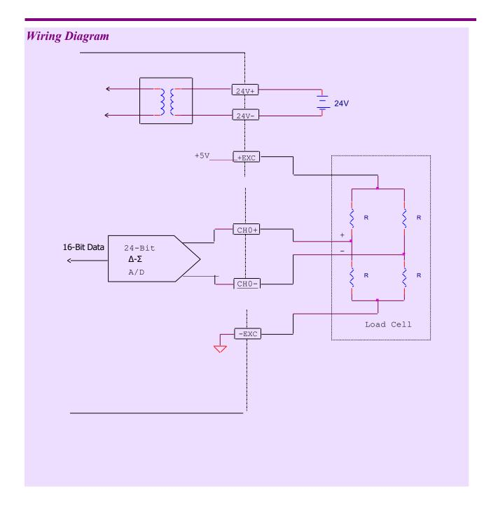
The raw conversion result is represented by a 16-bit signed value. After setting the full range engineering value and perform the zero and full scale calibration procedure, the system will automatically convert the raw conversion reading value into engineering weight value for user application.
