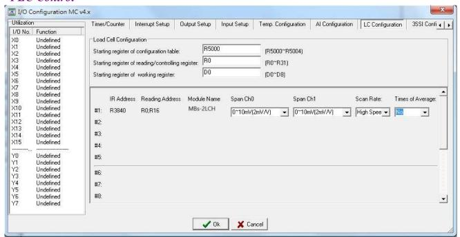
Before MBs-2LCH module can be working, the configuration of the module should be set by the Winproladder software tool. The picture shown at above is the I/O configuration page for "LC module" setup.
