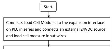
Execute the WinProladder and configure the load cell configuration table address, the register address, and working register in load cell configuration windows, then you can read the weight measurement value form register directly.
