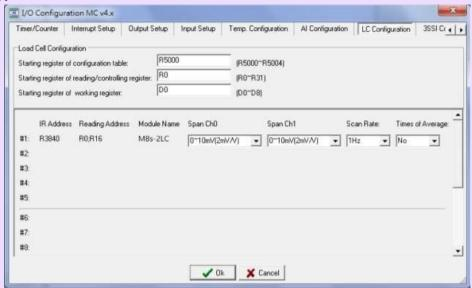
Before MBs-2LC module can be working, the configuration of the module should be set by the Winproladder software tool. The picture shown at above is the I/O configuration page for "LC module" setup.
