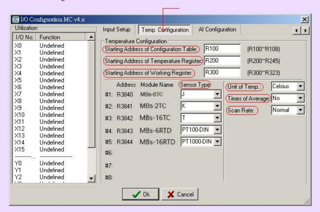
The user need to assign a starting register of a contiguous register area for holding temperature reading value and areas for storing the configuration table and working scratchpad and define the sensor type, unit of temperature, scan speed and samples for average. Please refer the advanced manual II for detail explanation.
