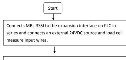
Execute the WinProladder and configure the 3SSI configuration table address and the data register in 3SSI configuration windows, then you can read the measurement value form register directly.
