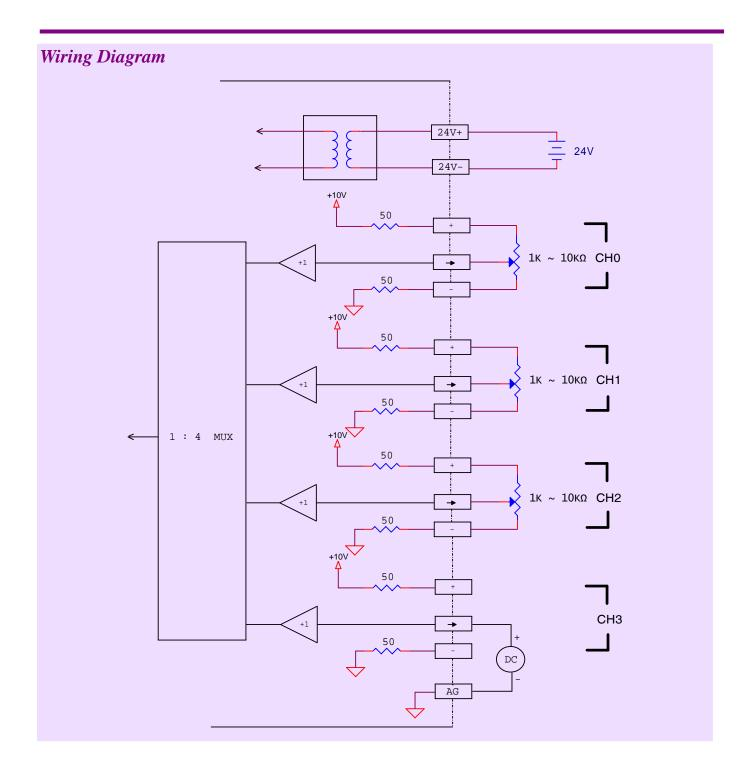
In the above sample wiring, the wiring of CH0 $\sim$ CH2 are for potential meter, while the CH3 is for  $0 \sim 10 \text{V}$  single ended voltage type signal. The internal serial resistors at upper or lower leg for each channel are for wire broke detection purpose. The too big or too low input value indicates the wire broke situation.
