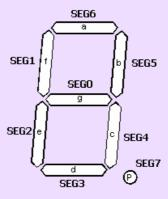
The driving signal of right most digit of display board is mapped to SEG0~SEG7 segment output and the next digit is SEG8~SEG15 while the left most one digit is SEG63~SEG56. One 7SG1 module can control 8 digits of seven-segment display.
