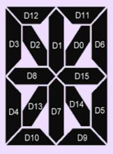
The D0~D15 of right most digit of alphanumerical display board is mapped to SEG0~SEG15 while the D0~D15 of the left most digit is mapped to SEG63~SEG48. One 7SG2 module can control 8 digits of 16-segment display.
