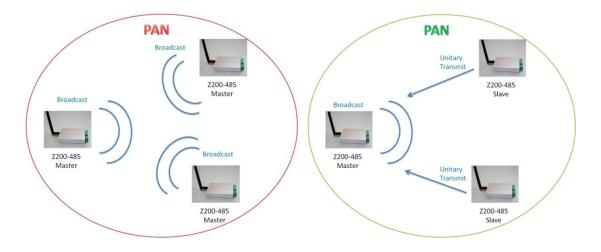
When a Master mode MBs-CMZBR sends RF packets, it broadcasts the packet to all the devices with the same PAN ID. On the other hand, when a MBs-CMZBR, as a Slave, sends data wirelessly, it only sends the data to the Master with a same PAN ID. In order for a Slave to work with a Master, user must pair each other. After successful pairing, the Slave will remember the Master's address and will be able to send RF packet directly to the Master.
