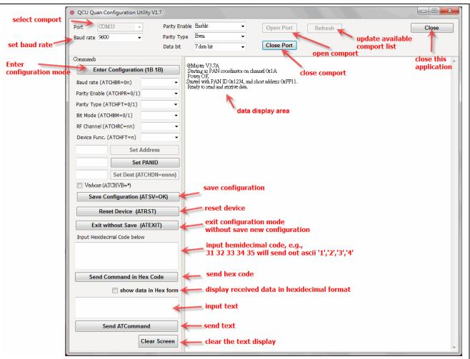
iii. In QCU, choose the correct COM PORT number and press "Open Port" button. Then the QCU is able to talk with the connected MBs-CMZBR.
