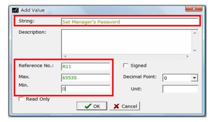
After setting the password values, press the button to add the value items under the Set Password menu as shown below.
