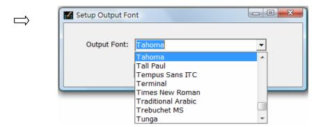
After selecting the desired font, press the button. The font on the PEP will be changed into the selected font. You can validate this with the [Off-line Simulation] function as shown below.
