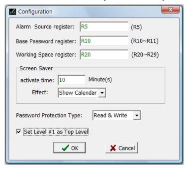
**X** Alarm Source Register: Set the address of the register storing conditions activating alarms. It is a 16-bit register. As shown in the example, the Alarm Source Register is R5, which means R5 is the register where the key values activating alarms are stored. When the values in R5 and the designed index are identical, the alarm activates. When the field is blank, there is no alarm.
