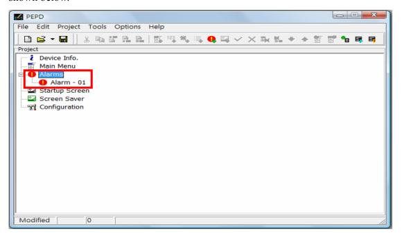
**Step 6:** Check the alarm configuration with [On-line Simulation] as shown below.
