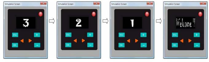
**X** If you want to enter the Main menu after running the startup screen once, set Cycle Count to 0. If you want to run several time, you can set the Cycle Count according to the desired times. The maximum is 10 Cycle Counts.
