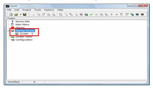
**%** The "0" in Screen-0 represents the first startup screen. There is space for up to 16 startup screens.
