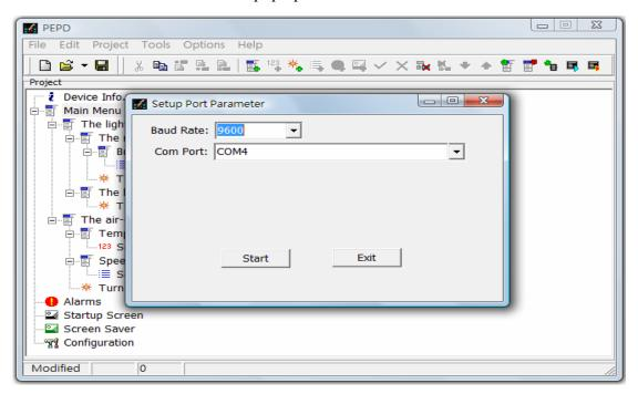
Step 4: After setting up the Baud Rate and Com Port, press the Start button. The [On-line Simulation] screen will pop up as shown below.
