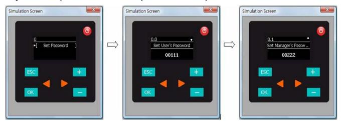
After setting the passwords, shut down the simulation and re-start the [On-line Simulation]. Before entering the menu page, you will be requested to enter the password. You must enter the correct password in order to access to the menu as shown below.
