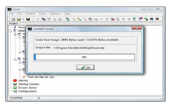
Step 3: After verify the compile result is OK, press the button and the Setup Port Parameter window will pop up as shown below.
