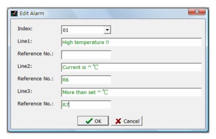
**%** In Line 2, the "^" symbol marks the display location of R6 content; and in Line 3, the same symbol marks the display location of R7 content.
