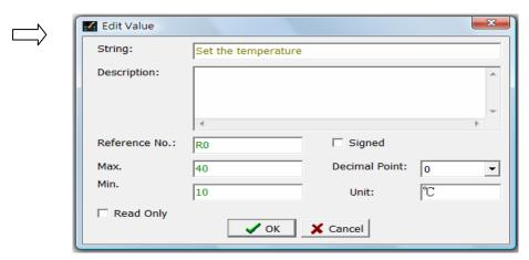
**\*\*** In this example, "R0" is the reference number corresponding to the PLC, i.e. the register assigned to save the value for Set the Temperature. The Maximum and Minimum values are 40 and 10 respectively. The temperature unit is °C.
