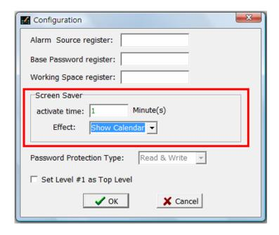
After setting the time and effect, press the button. You can check the settings with [Off-line Simulation] as shown below. When "None" is selectd, though no screen saver action will be activated when the idling time is up, you still need to enter the password, if enabled, to re-enter the normal screen.
