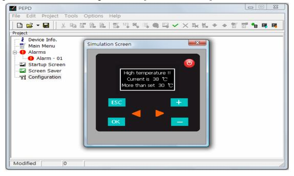
**X** You can also check the alarm configuration with [Off-line Simulation]. When an alarm is set, the icon will appear on the [Off-line Simulation] screen. Click the icon to select the "Index" for running "Alarm Trigger" as shown below.
