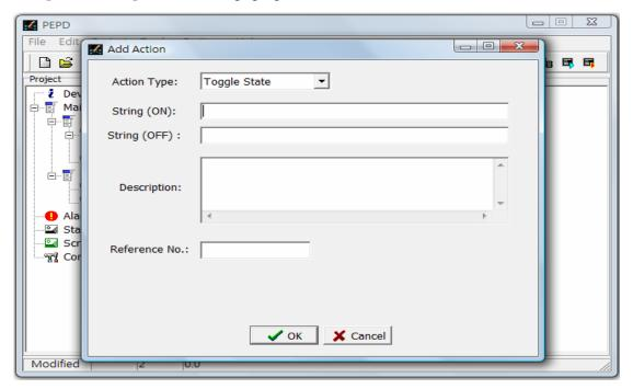
**\*\*** In the Action Type item, select Toggle State for Light Switch. You can enter the action strings according to the information in the following example. According to the example, when the action is activated, "Y0" will be the reference number corresponding to the PLC, and the actions On and Off will be displayed alternately.
