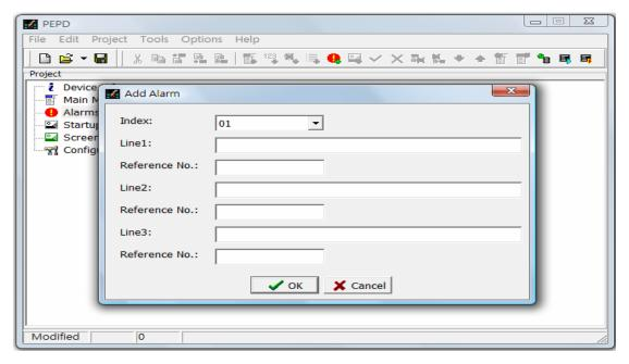
Mex: Users can set any number from 01-64. When the value in the Alarm Source Register in Configuration is identical with the Alarm No., the alarm message of the corresponding Index will be activated. Therefore, the maximum number of alarms is 64.
