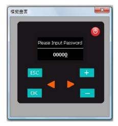
**\*** The main difference between the operator password and supervisor password is that the former allows users to access the menus but not the system functions when the supervisor password protection is enabled. In this case, users need to use the supervisor password to access the system functions.
