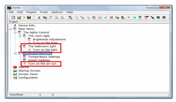
**%** In this example, the reference numbers corresponding to the PLC are: "Y0" for The Room lights (On/Off), "Y1" for The Bathroom lights (On/Off), and "Y2" for The Air-con Switch. As shown below.
